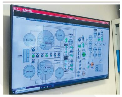
VTSCADA system, complete with graphics for screen displays, motor controls, levels, trending, and alarming. This not only provided local system controls but also enabled remote monitoring and control.
